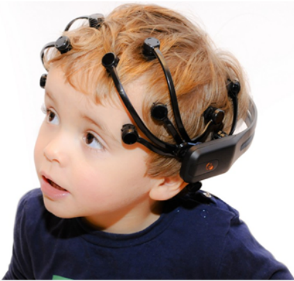
Fig. 1: Brain signal recording using Emotive EEG headset, 10-20 electrode positioning (image courtesy: www.emotive.com & https://lucid.me/blog/wed-love-try-emoativ-epoc/ )
