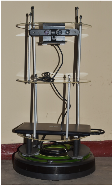
Fig. 1. Mobile Robot System: iRobot Create 2 base, PrimeSense 3D sensor and mini-laptop.
